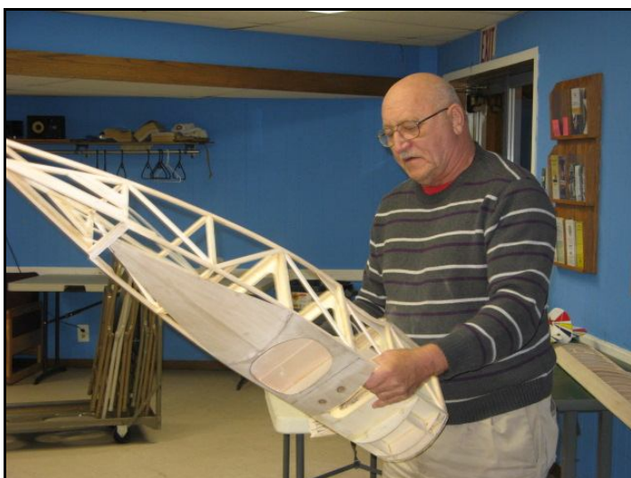
Stan Zdon showed his Balsa USA Fokker Triplane. The die cutting was excellent for his kit. The instructions have you build the wings first. The top wing will be permanently attached to the middle wing. He plans to use an OS Surpass 155 4-stroke for the engine. Ailerons only on the top wing, but they are big! He is using graphics from www.callie-graphics.com . Stan estimates the model will weigh 14-15 lbs when done.
