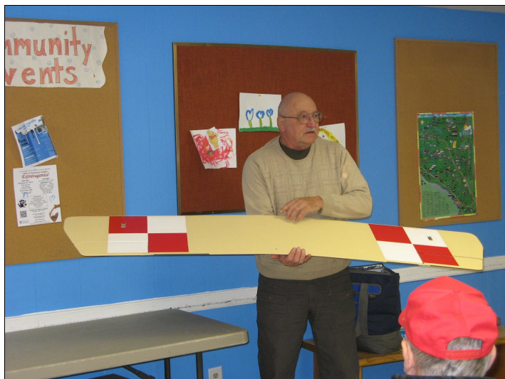
Stan Zdon brought in the lower wing and the tail from his Sopwith Pup. It is 1/4 scale plane built from a Balsa USA kit and will be powered by a Saito 150.
